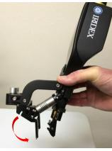
4. Release the eye-safety filter plate from its storage detent position.
